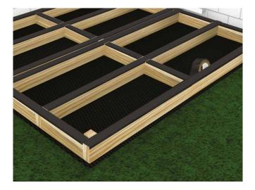
The maximum recommended space between Joist rows depends on the angle at which you intend to lay your boards in relation to the Joists, but should **never exceed 40cm**, please see diagram. Apply Deck Tape to the top surface and cut ends of the timber joists to protect them from moisture.
