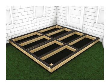
2 Starter Clips need to be fixed to the end of the Joists before laying the first Board. Place these at the end of each Joist, leaving a gap of 15mm between the wall and the Starter Clip to allow for expansion.
