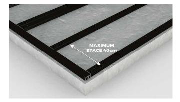
**1** Boards must not be laid directly on the ground but should be fixed to the Joists. The maximum recommended space between Joist rows depends on the angle at which you intend to lay your Boards in relation to the Joists, but should **never exceed 40cm**, please see diagram Composite Joists should be screwed into the concrete base.
