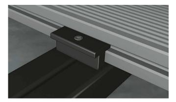
**5** Slot T-Clips into the groove along the side of the Board and screw them into the supporting Joists with the screws provided, using one T-Clip for each supporting Joist. We recommend you use our Stainless Steel Wood Screws offering increased wear and less corrosion. **T-Clips will leave a 7mm gap between Boards.**
