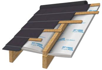
The product should be installed with the stitched edge positioned towards the highest point of the roof with the built-in 100mm overlap nearest the eaves/gutter.
