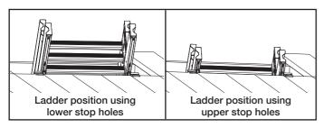
**9** Check the ladder angle against the safety label or refer back to Deployed Requirements on page 2.
