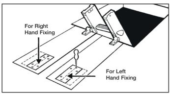
Place the spring housing (E1) in position over the holes ensuring the arm points AWAY from the loft opening (with slot in cover on the left-hand side).
