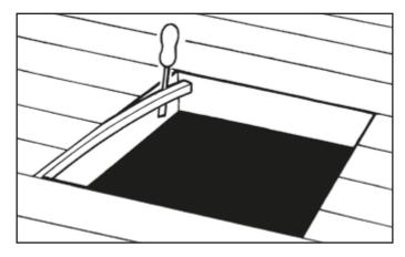
**1.4** Screw hinges (F5) to one edge of the trapdoor using 20mm (3/4") wood screws (F6).
