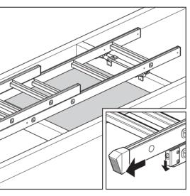
**10.** Using a suitable ladder, gain access to the loft and position the loft ladder centrally across the loft opening with the pivot assembly resting squarely on the trapdoor surround. To help with access, release the locking catch on the end of the top ladder section and slide the bottom section down the ladder.
