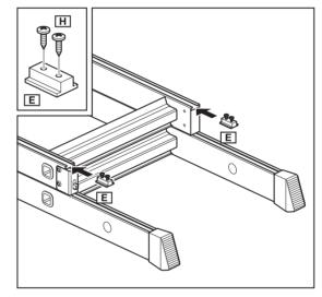
**7.** Loosely insert 12mm screws (**H**) into both stops (**E**) and slide into the top ladder section.
