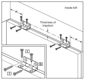
**1.** Attach hinges to trapdoor and opening. Drill 2mm pilot holes, attach hinges (G) to trapdoor and surround using  $8 \times csk 20mm$  screws (I). Note: The trapdoor will attach to the same side of the opening as the ladder (Trapdoor is not supplied).
