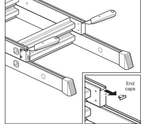
**6. Prepare the loft ladder.** Using a sharp knife, carefully cut along the grooves and remove both end caps. Keep end caps for later use.
