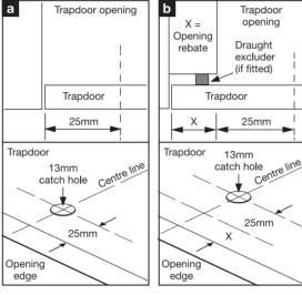
**2. Mark and drill catch hole in trapdoor.** Mark the centre line onto the opening edge of the trapdoor. Measure 25mm in from the opening edge of the trapdoor and drill a 13mm hole (a). Note: If the trapdoor opening has a rebate 'X', add this distance to the 25mm (X + 25mm) (b).
