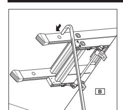
**15. To lower ladder.** Insert the pole (**B**) into the round hole on the bottom ladder section and **carefully** pull down until top section rests on top stops. **IMPORTANT: Control the movement of the ladder at all times. DO NOT allow ladder to fall under its own weight.**
