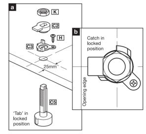
**3.** Assemble the catch. Assemble the catch onto the trapdoor ensuring the 'tab' on the catch barrel and the catch are positioned as shown (a). Note: Only fix the retaining washer (C3) using the 12mm screw (H) once correctly positioned as shown above (b).
