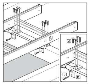
**11.** Ensure both pivots (**D**) are spaced as far apart as possible (up against the glides). Use a bradawl or small drill to start the screw holes, attach the pivots to the trapdoor surround using  $10 \times 25$ mm screws (**J**).
