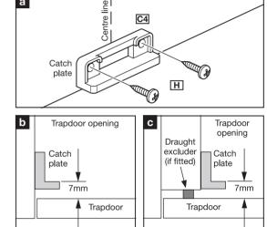
**4. Attach catch plate.** Find and mark the centre line onto the opening end of the trapdoor surround. Allow a 7mm gap between the top of the catch plate and the trapdoor (**b** or **c**). Attach the catch plate (**C4**) to the trapdoor surround using  $2 \times 12$ mm screws (**a**).
